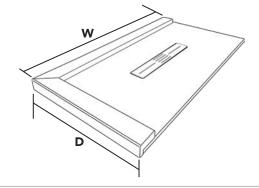
\*Represents the min or max depth and width of base when not trimmed. The base can be cut in the field up to 4" in width away from either side of drain on center drain models and up to 4" in width away from side opposite drain on end drain models or up to 2" in depth away from the drain to accommodate different dimensions.
