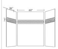
Wall can be trimmed to size in the field. Recommended height for bottom panel is 60" - 72".
