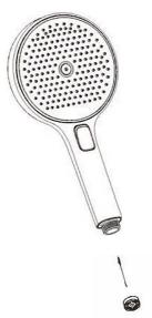
2. Screw on the hose tightly and test for leakage.
