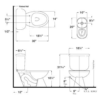
This toilet is designed to rough-in at a minimum dimension of 305mm (12") from finished wall to C/L of outlet. Supply not included with fixture and must be ordered separately. Dimension shown for location of supply is suggested. For additional information refer to installation instructions supplied.
